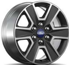
18" Six-Spoke Machined-Aluminum with Magnetic Painted Pockets (Incl. in XLT/Lariat Sport Appearance Pkgs.) – 64R
